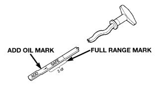
Never operate the engine with oil level below the "ADD" mark or above the upper "SAFE" mark.
